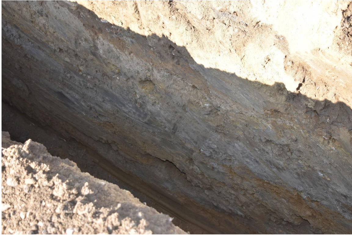
Photo 11: The soil profiles consisted of a mix of silt and clays overlying glacial till. View of Trench 1.
