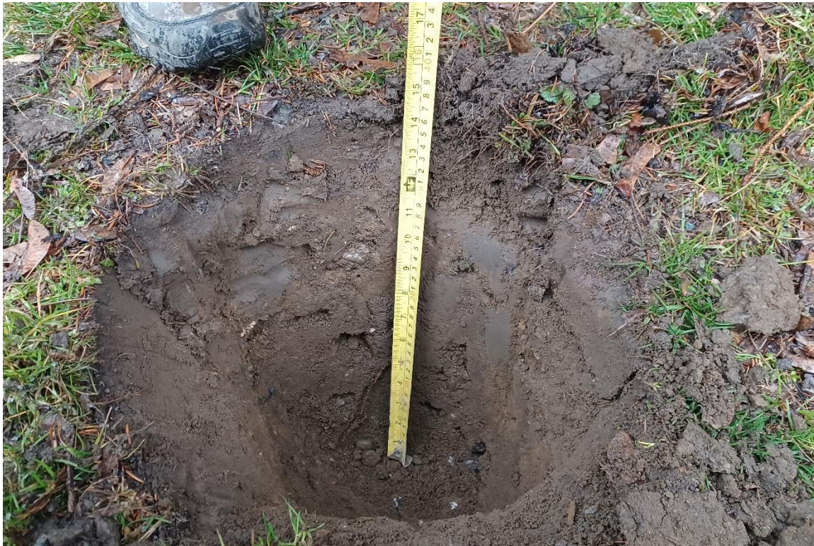
Photo 7: The shovel tests identified fill soils, mixed with plastic, rebar and dense gravel. View of ST 5.
